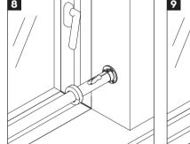
Slide the Sockets and covers onto the rai Insert the screws and tighten the grubscrew
