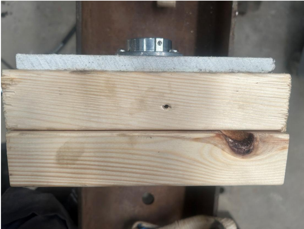
Plate 1 – Detail View of Sample Installation onto Substrate – Timber Frame
