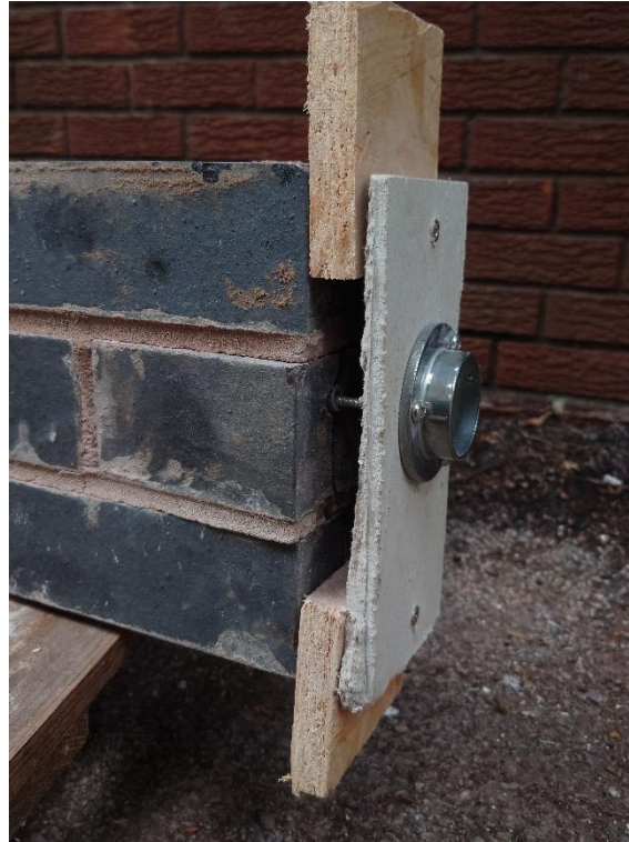
Plate 1 – Detail View of Sample Installation onto Substrate – Clay Brickwork
