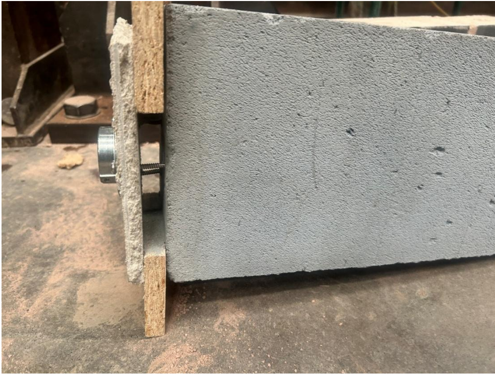
Plate 1 – Detail View of Sample Installation onto Substrate – AAC Blockwork
